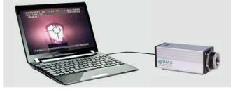
The DSR 10NF/DSR 10NFV are equipped with galvanically isolated RS-485 interface which allows parameterizing and software evaluation even in bus systems. The black body temperature with emissivity calculation, the colour temperature and the optical thickness are readable.
