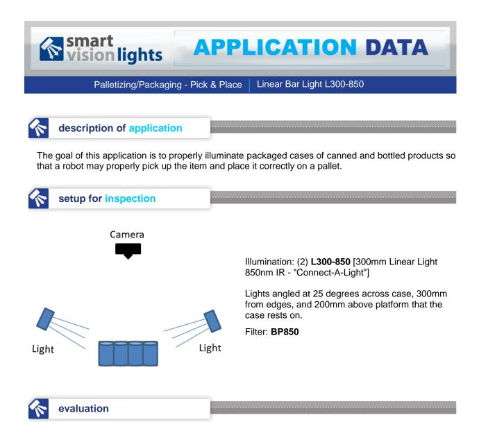
Problem – product variation and palletizing. Products could be 6 or 18 packs. Each pack could be wrapped with any color package with logo or marketing material. So the goal was to illuminate the 6-18 pack so the robot could pick. IR was used to reduce the color issue as color could cause low contrast. It was important to test with the lights pointing at different angles. We found that low angle lighting provided the best results and two lights were used to achieve the desired illumination level.
