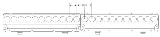
The spacing between the high current LED's is the same between lights as in an individual light. The LED's remain equally spaced between lights. When lights are connected together placing lights end to end there is no uniformity difference measured at a 300mm (12") working distance or further.
